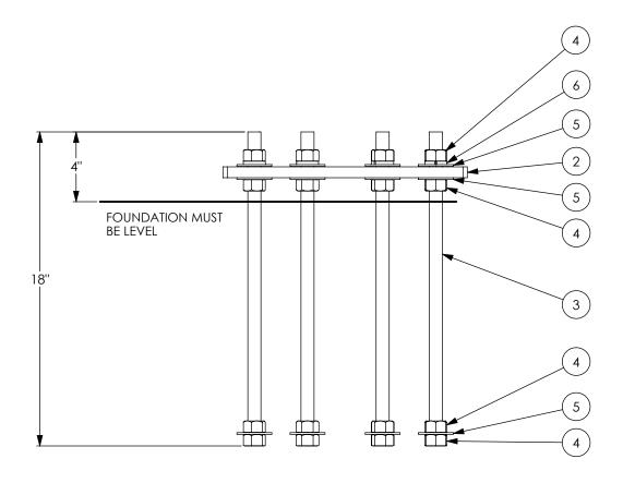
On one end of each rod attach a flatwasher sandwiched between two hex nuts. Attach the the other end of the rod to the wood template as shown in the diagram. The wood template will help the keep the rods aligned. When pouring the concrete keep the top 4" of thread clean.
