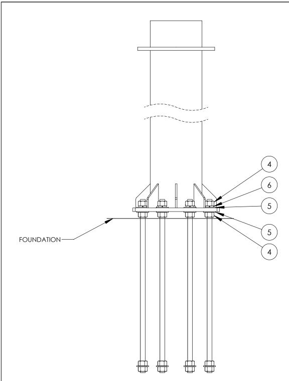
Remove the wood template after the concrete has cured. Clean the exposed threads and turn a nut all the way down to the top of the concrete on each rod. Set the pedestal and tighten hardware. See the drawing above.
