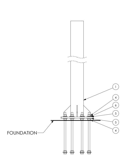
Remove the wood template after the concrete has cured. Clean the exposed threads and turn a nut all the way down to the top of the concrete on each rod. Set the pedestal and tighten hardware. See the drawing above.
