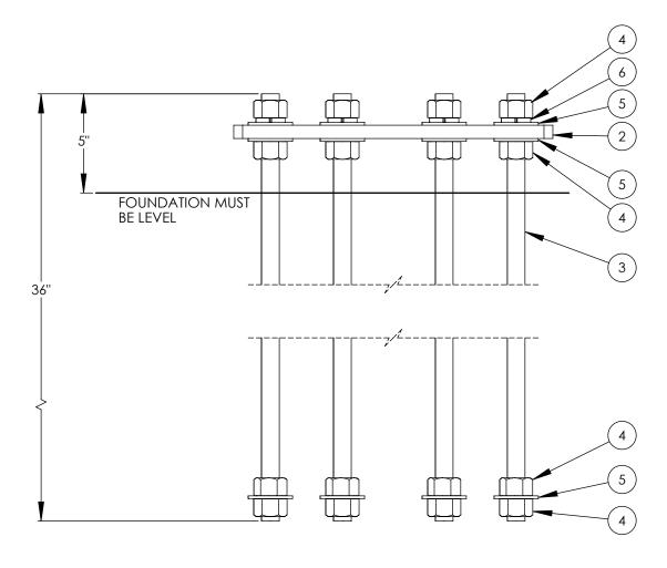
On one end of each rod attach a flatwasher sandwiched between two hex nuts. Attach the the other end of the rod to the wood template as shown in the diagram . The wood template will help the keep the rods aligned. When pouring the concrete keep the top 5" of thread clean.
