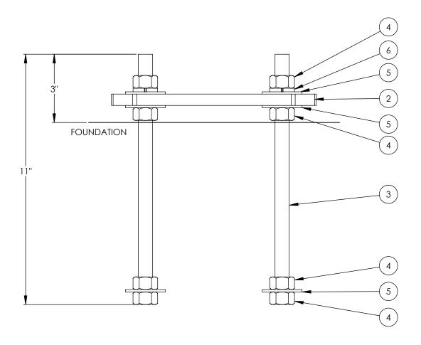
On one end of each rod attach a flatwasher sandwiched between two hex nuts. Attach the the other end of the rod to the wood template as shown in the diagram. The wood template will help the keep the rods aligned. When pouring the concrete keep the top 3" of thread clean.
