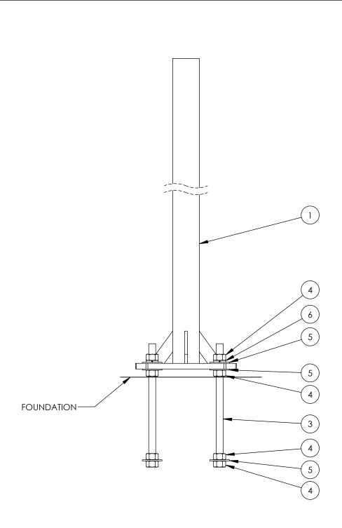
Remove the wood template after the concrete has cured. Clean the exposed threads and turn a nut all the way down to the top of the concrete on each rod. Set the pedestal and tighten hardware. See the drawing above.
